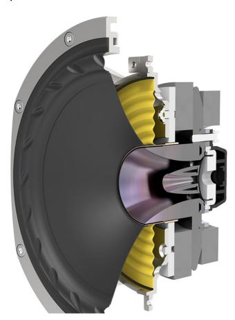
This is a superbly engineered driver supported via a cast aluminium chassis and bearing a massive 'flux-focusing' magnet system. Within the motor, Fyne Audio engineers have placed a pole piece incorporating an efficient heatsink allowing high power output. Further heat dissipation is provided by a
